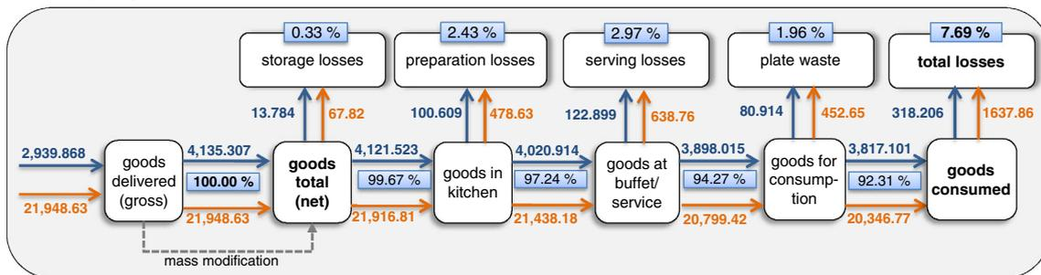
**Fig. 5.** Simplified material flow analysis (MFA) of FSC in a food service company. Upper box (a) shows result of company A, lower box (b) of company B. All blue values are quantities in kg, all orange values are cost prices (including value added tax) in CHF. Loss refers to total loss including avoidable and unavoidable losses. The term 'gross' is used for unprepared food; all others without denotation are net weights.
